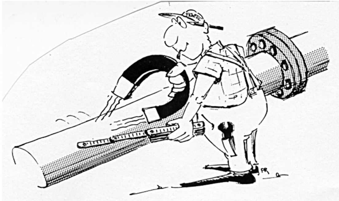
Principle of the electromagnetic flowmeter (EMF)
